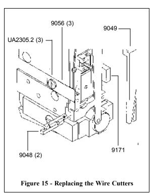
After replacing or installing new parts, rotate the Drive Pulley manually to check for free movement.
