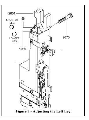
leg. Once the desired length has been achieved, tighten the Binder Screw and the Wire Guide Spring Bracket Screw. At this point, the left leg should be approximately one half the width of the crown.
