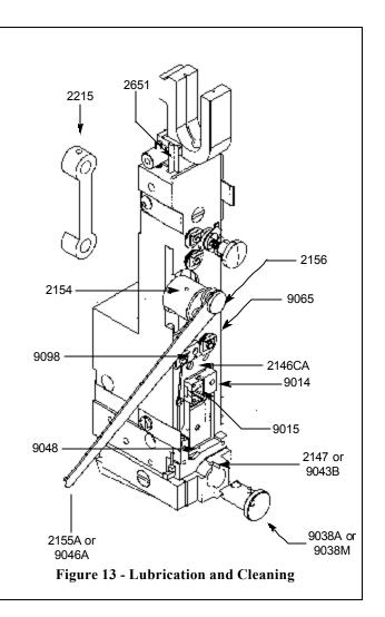
In addition to proper lubrication, routine cleaning is important for the maintenance of your 26/26D Head. The entire Head should be torn down and rebuilt every three months and the following areas should be cleaned once a month:
