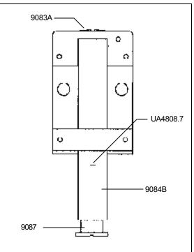
Figure 11 - Adjusting Clincher Points
