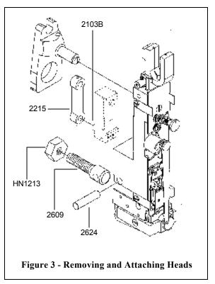
Verify that the Driver Shaft Connecting Link (2215) is squarely engaged with the Crank Pin on the stitcher machine and the Driving Slide Pin (2103B) on the stitcher head and that they do not bind. Secure this position with the Bonnet Stud Nut. (HN1213)
