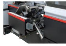
Install the special drain for glue run-off. The PUR tank and drums are teflon coated so that the remaining glue can be easily peeled off after cooling.
