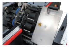
The application drums and back spinner lift and latch to provide easy access for cleaning of the tank.
