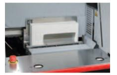
A rigid clamping system holds the book block firmly in position during the milling and nipping process to produce a quality finished book. The safety curtain ensures risk-free operation.
