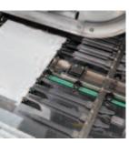
After transport to the nipping section, the cover is registered precisely with the fore-edge guide and tail-edge positioning guides.
