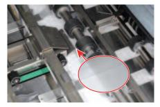
The scoring width and position are automatically set-up according to book block thickness and cover registration. Scoring is performed on thick covers for professional binding with sharp, square spines and hinge scores.
