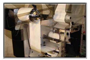
Run 3" wide labels on the standard KR540. Even wider labels are possible using the optional 5" wide label kit.
