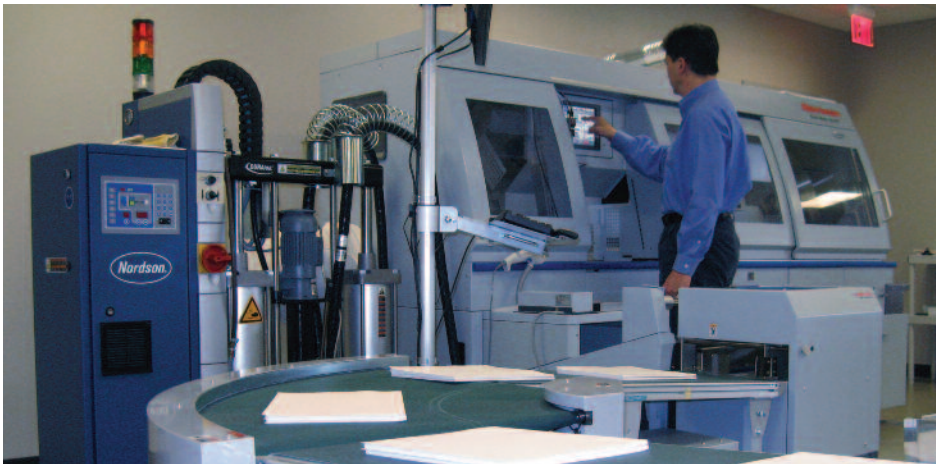
Greg Nakanishi, Standard senior technical service engineer performs a changeover on the Horizon BQ-470PUR.
